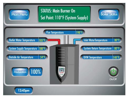
When the ON/OFF switch is turned to the ON position, the first screen visible on the LCD display will be the Home Screen. This screen displays the current status of the Crest boiler. The following items can be viewed or interacted with on the Status Screen:
