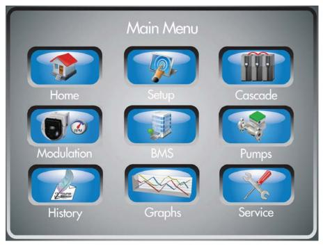
The Main Menu Screen allows navigation to nine (9) additional screens which are used to set temperatures, operating conditions, and monitor boiler operation. These screens are as follows:
